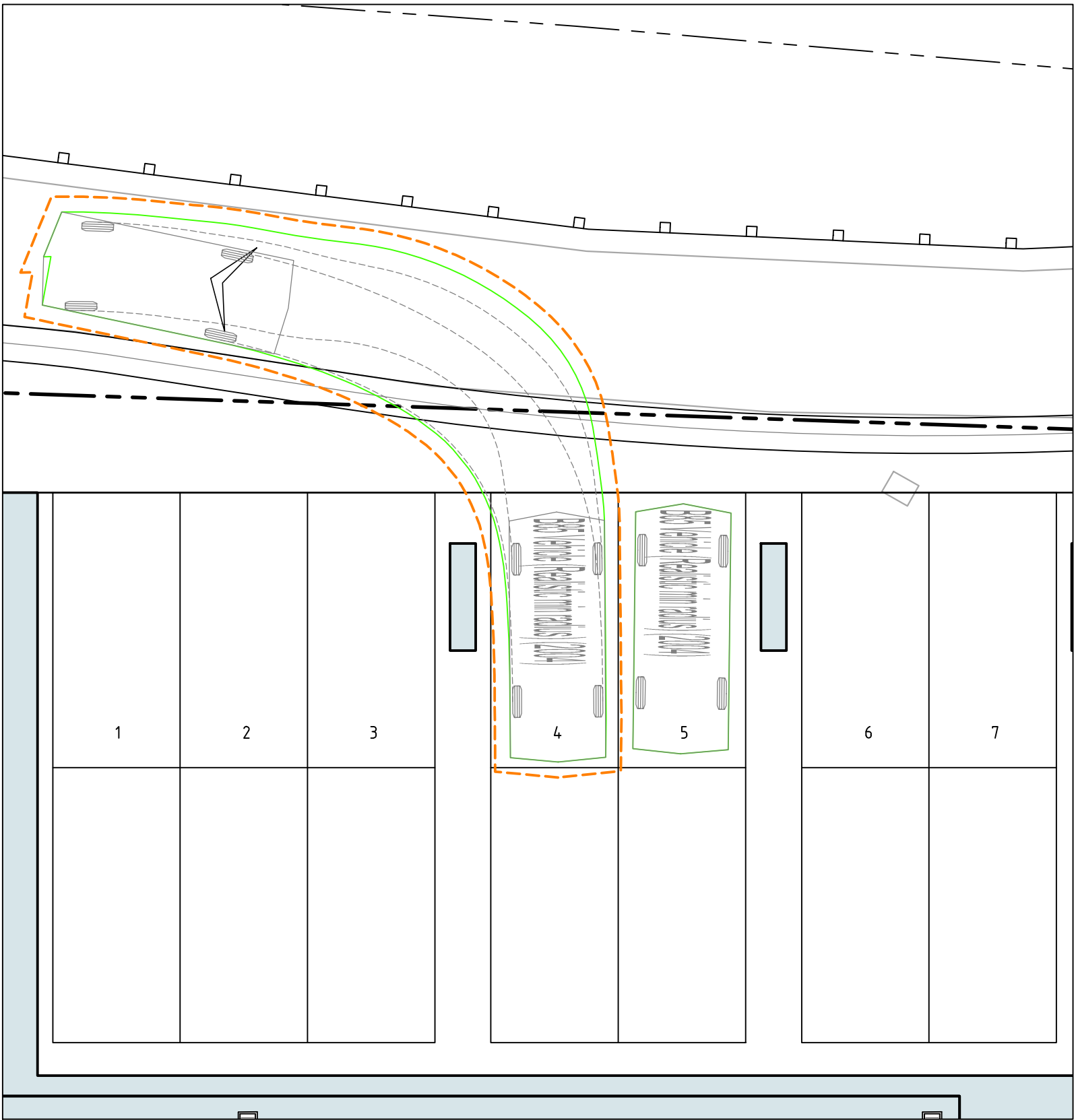
PARKING BAY 4 FORWARD EXIT B85 SCALE 1:100
