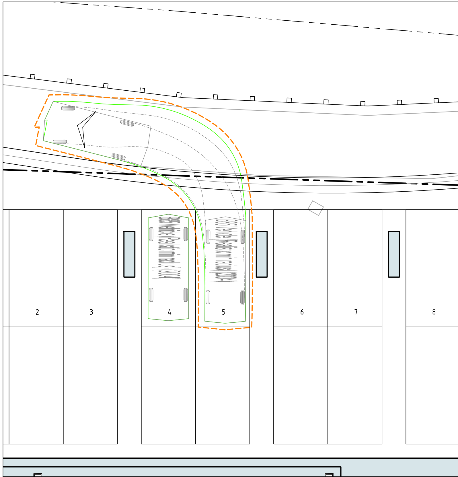
PARKING BAY 5 FORWARD EXIT B85 SCALE 1:100
