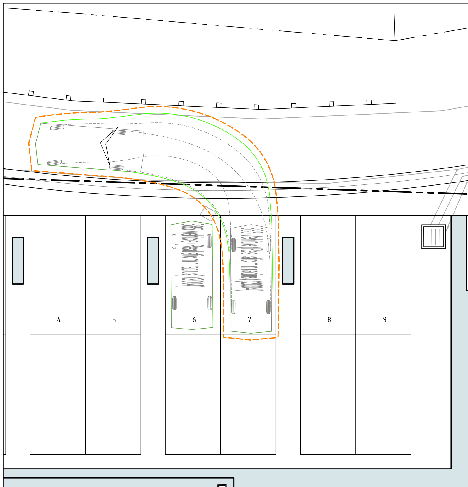
PARKING BAY 7 FORWARD EXIT B85 SCALE 1:100
