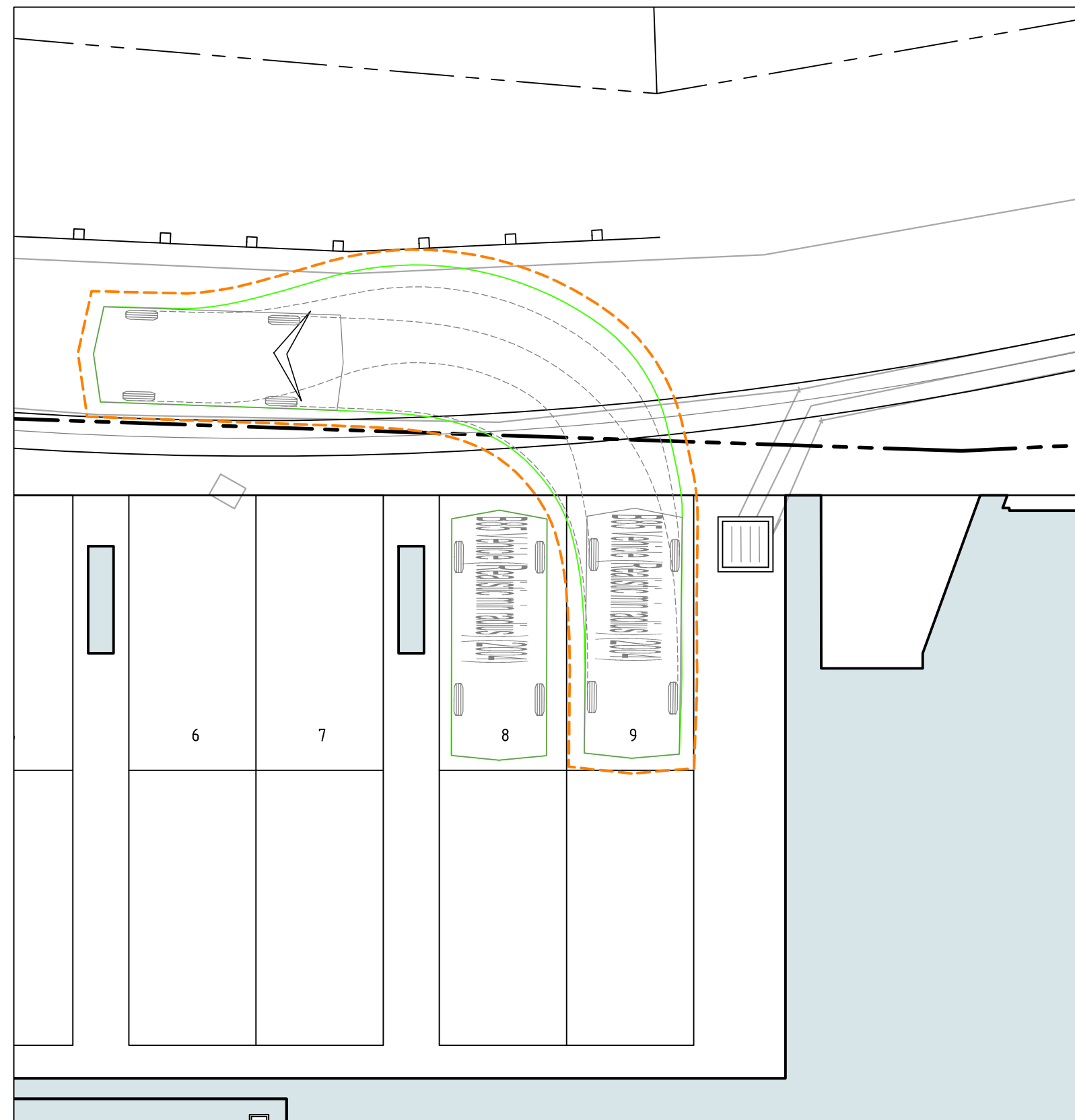
PARKING BAY 9 FORWARD EXIT B85 SCALE 1:100
