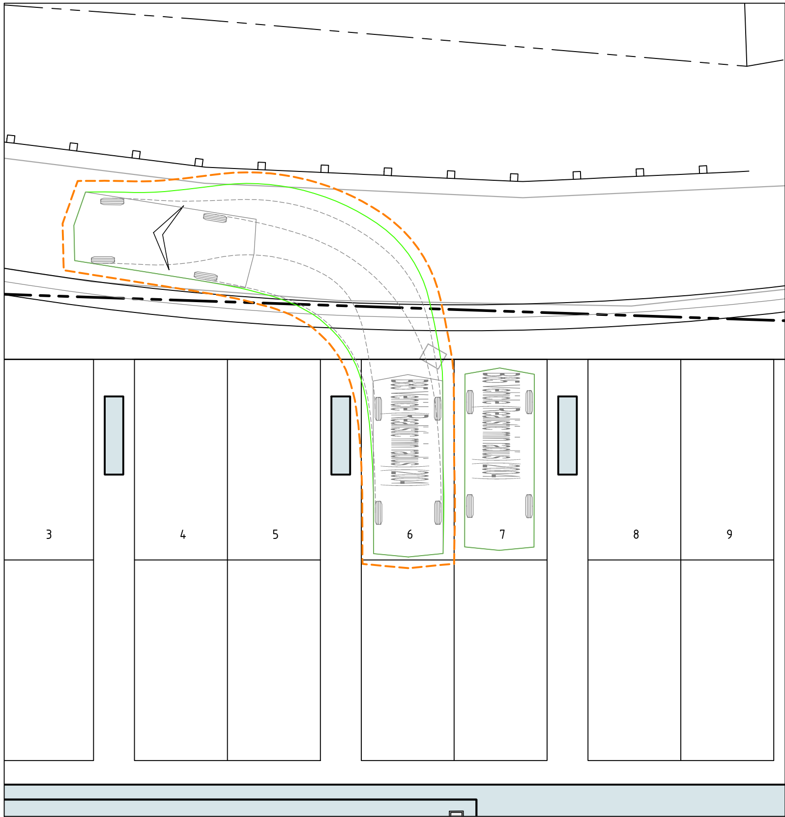
PARKING BAY 6 FORWARD EXIT B85 SCALE 1:100
